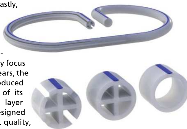
Internal configurations of different designs used on wound drain and surgical tubing no longer require separate sections to be extruded, then joined. The Guill reciprocating head design produces various profiles within the tubing in a constant production run
