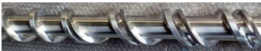
Pic. 1: 22 L/D long barrier part for best melt quality
